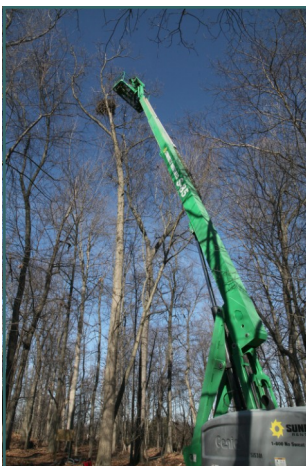
Lift used to install camera
